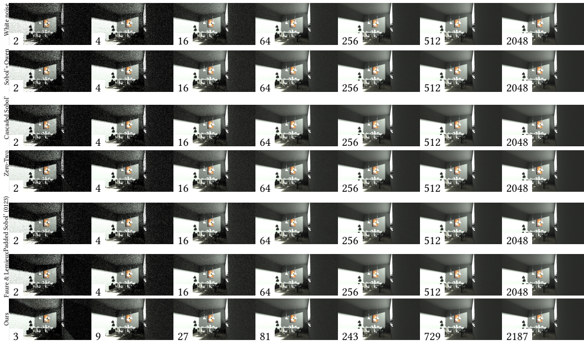
Figure 13: 10-d rendering with one bounce of indirect lighting, 1 mostly occluded light source, diffuse and glossy materials. Direct lighting with a multi-sample MIS estimator. Indirect bounce samples the material definition.
