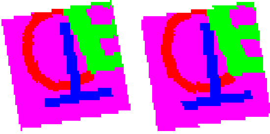
Fig. 12: Bijective rotation of the same image and the same target angle ( 10^\circ ) with CDLR but we choose to minimize with respect to L_\infty + \lambda L_c (a) with \lambda = 0 , (b) with \lambda = 70 .
