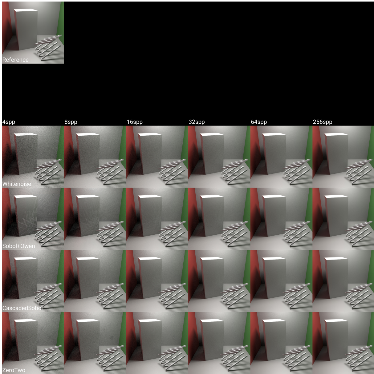
Fig. 6. Rendering 1 bounce indirect lighting with 6-dimensional samples. Cornell box with a high frequency sub-pixel texture pattern on the back wall. Highly discontinuous integrands.
