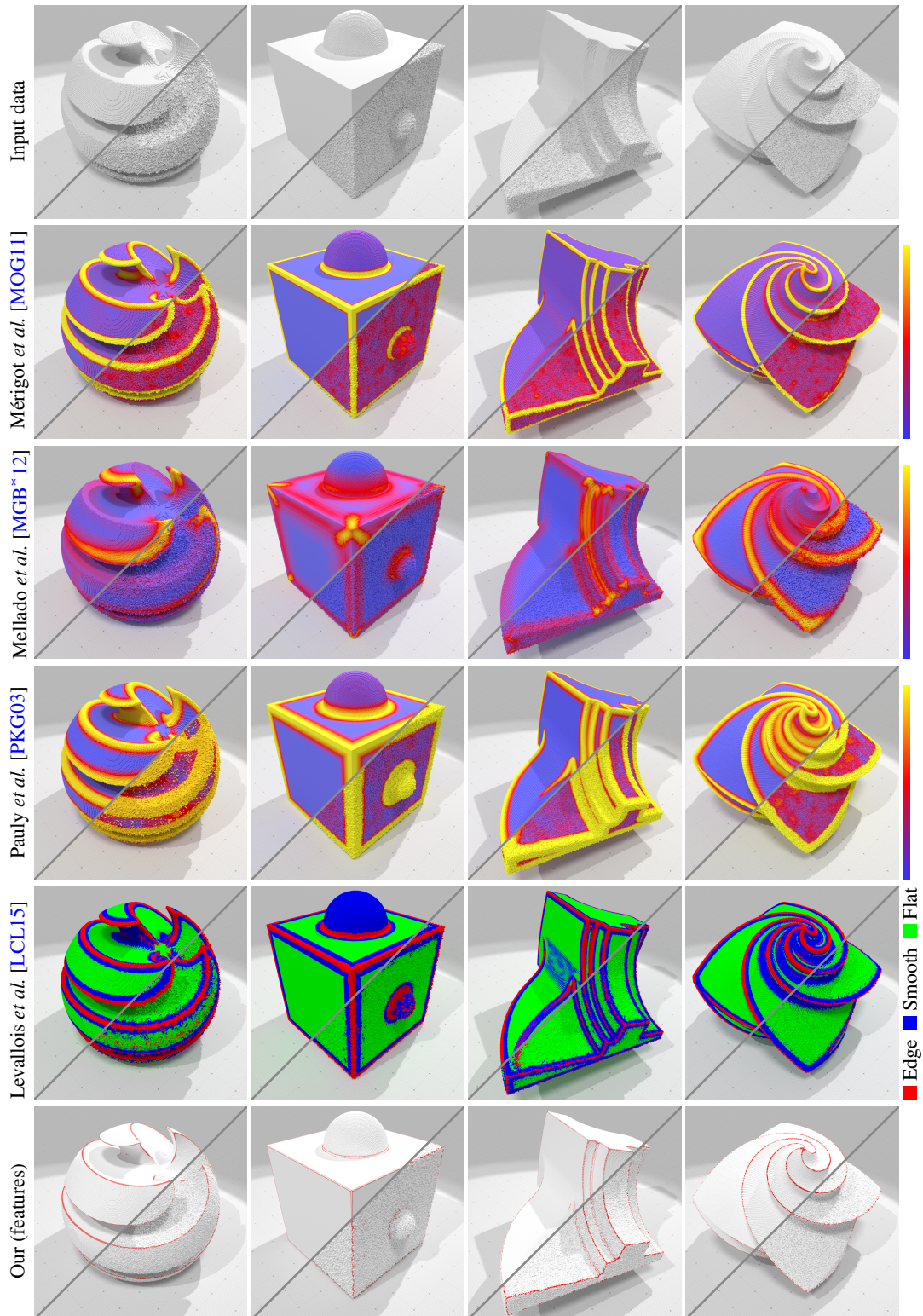
Figure 4: Evaluation of feature detectors on perfectly digitized shapes. SharpSphere : 256^3 voxels, CubeSphere : 200^3 voxels, Fandisk : 512^3 voxels, OctaFlower : 512^3 voxels. Parameters used for [MOG11]: R_1 = 10 , r_1 = 10 , T = 0 . Parameters used for [MGB*12]: r_{min} = 5 , r_{max} = 25 . Parameters used for [PKG03]: r_{min} = 5 , r_{max} = 25 , \tau_{max} = 0.01 . Parameters used for [LCL15]: r_{min} = 5 , r_{max} = 20 . Parameters used for our approach: \alpha = 0.1 , \lambda = 0.01 , \epsilon = [2, 0.25] with integral invariant normal vector estimator with radius 8. Bottom-right parts of images correspond to the results with the same parameters and noise level k = 0.5 .
