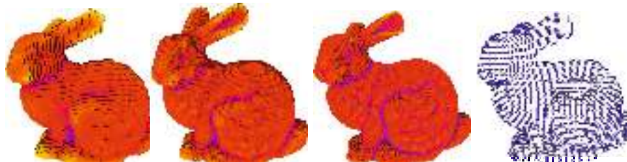
Fig. 7. (Left) Mean curvature mapped on “bunny” at different resolution using \hat{H}_l^* (yellow color is the highest curvature, blue the lowest). (Right) First principal direction on “bunny” using \hat{k}_l^* estimator.
