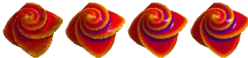
Fig. 7. Illustration of mean curvature computation on “OctaFlower” (digital domain of 130^3 ) using mipmap approximation with different levels: l_3 , l_2 , l_1 and l_0 ( i.e. no approximation).
