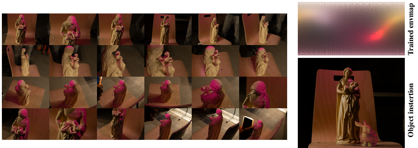
Figure 9: Trained environment map on a real scene. The geometry was reconstructed using Colmap [SF16] using around 50 photographs (24 are shown here). Two lights are used to illuminate the scene: a yellow-white, and a magenta light, which appear on the resulting environment map.
