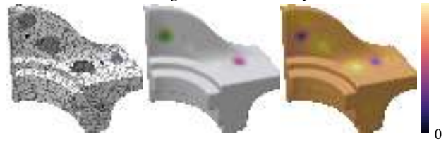
Fig. 9. Gaussian process scalar field inference using the kernel derived from the eigenfunctions of the \Delta_\varphi operator. Regression is performed by building a Gaussian process using the kernel Eq. 26 from scalar data (left) as in Sec. 3.2. The mean field of the regression is plotted in the middle and the variance field on the right. One can observe that the variance of the prediction is lower near the data points and is highest at locations where the uncertainty of the underlying GPIS is maximum.
