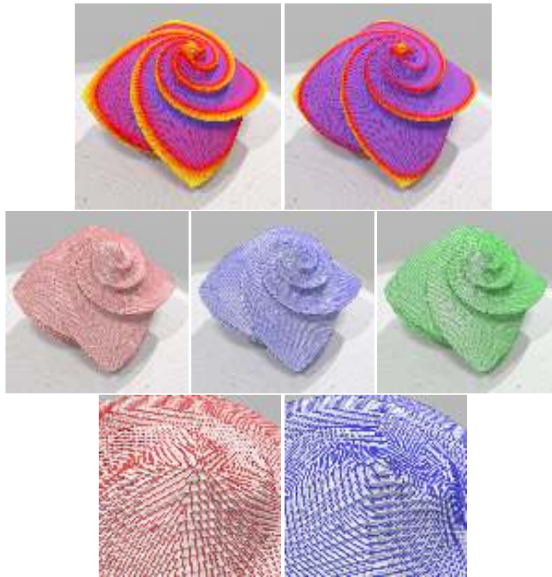
Fig. 1.9 Integral invariant based differential estimators on a digital surface ( 256^3 OCTAFLOWER shape). From left to right, mean curvature, Gaussian curvature, first principal direction, second principal direction and normal vector field (zooms in third row).
