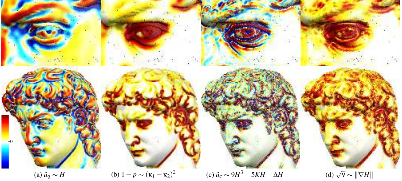
Figure 2: Geometric features: obtained from local algebraic sphere regressions performed on 2 million unstructured points (dark dots are due to the splats rendering). We summarize the relevant differential properties that are asymptotically linked to each of them by the symbol \sim . (a) The quadratic parameter is related to the mean curvature H (Theorem 1). (b) The deviation of the Pratt's norm from 1 defines an anisotropy measure (Proposition 1). (c) The constant parameter involves 4 th order derivatives which highlights fine surface variations (Theorem 1). (d) The squared root of the geometric variation [MGB*12] is related to the norm of the mean curvature gradient involving 3 rd order derivatives (Proposition 2).
