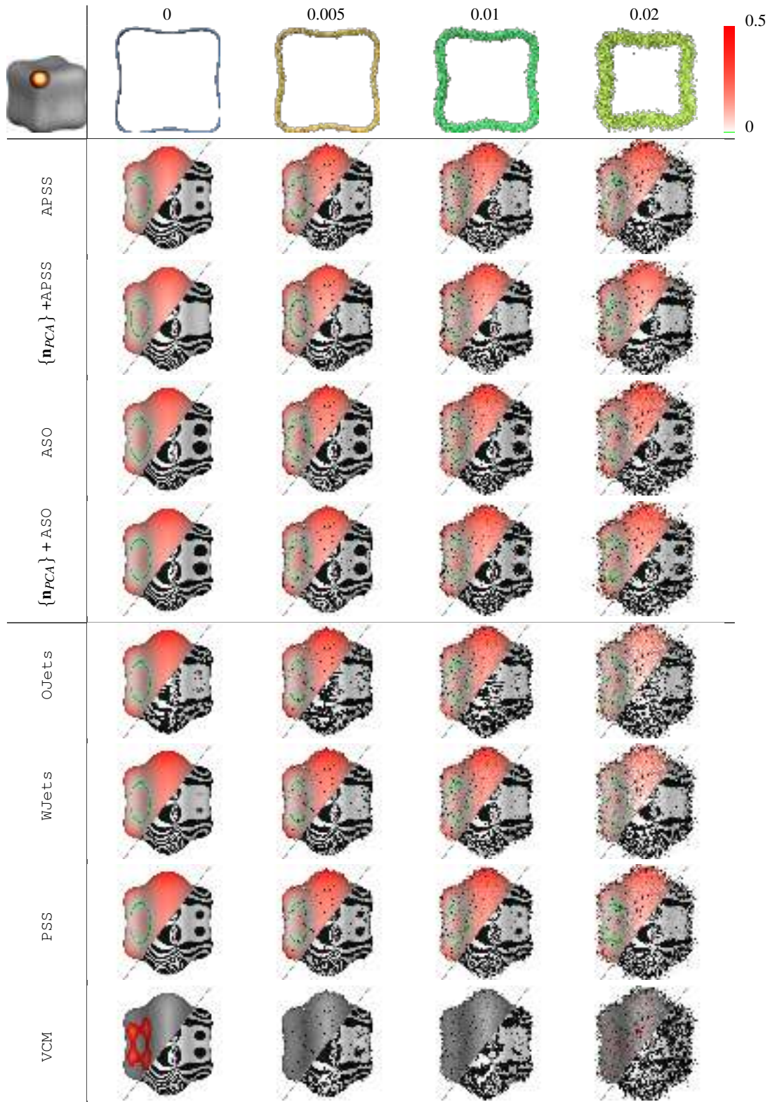
Figure 5: Stability with respect to noise on the positions: we evaluate the absolute value of the mean curvature and the corrected normal vectors for various noise level (Gaussian noise with standard deviations in \{0, 0.005, 0.01, 0.02\} ). Curvature measures are displayed using a white-red colormap with a green highlight for the zero-curvature values (grey values correspond to quantities outside the [0 : 0.5] range). To illustrate the smoothness of the corrected normal vectors, we consider a pure reflective material with a zebra like environment map to approximate isophotes.
