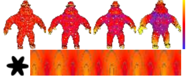
Figure 2: Top : Mean curvature using Eq. 6 for different ball radii: 4, 7, 14 and 30. Bottom : 2D flower and curvature values on its boundary using Eq. 5 (x-axis) for a range of decreasing ball radii (y-axis, from top to bottom). Curvature values are mapped from blue (lower) to yellow (higher), discrete gray lines illustrate curvature isovalues.
