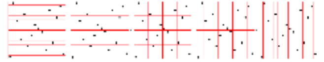
Figure 2: Illustration of dyadic partitioning, applied on first 16 points of Sobol LDS, dimensions 1 and 2 (all five sub-figures show exactly the same point set). Each partition of size 1 \times 16 , 2 \times 8 , 4 \times 4 , 8 \times 2 and 16 \times 1 contain exactly 1 sample.
