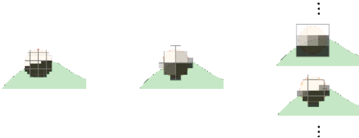
Fig. B.5.: Here are the three approaches we used to evaluate the integrand. ( left ) is the naive approach, where we sum all the digital points that are inside the integrand domain ( middle ) shows the hierarchical decomposition of the ball, thus limiting the number of texture probes to do. ( right ) illustrates the dynamic approach, we probe the textures at a higher resolution and we refine it at each frame until we reach the finer level.
