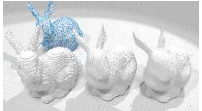
Fig. 13. Voxel upscaling: starting from a low resolution Bunny object ( 64^3 ), we can reconstruct its surface (blue piecewise smooth surface) and use it to upscale the input object to 256^3 and 512^3 resolutions (middle and right).
