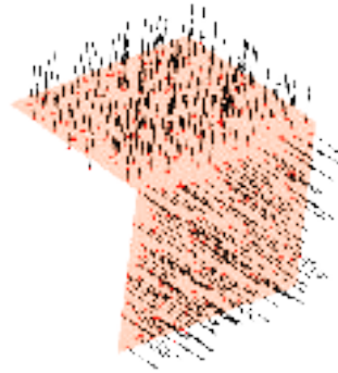
Figure 4: Planes intersection with ground truth normals used as synthetic model to evaluate our algorithm.
