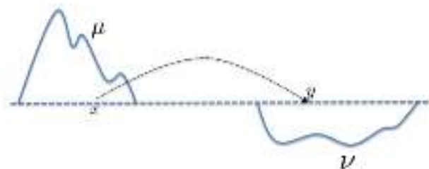
Figure 1. Graphical representation of the mass transportation problem. The minimal effort cost to transport one measure into the other defines the OT distance between \mu and \nu .
