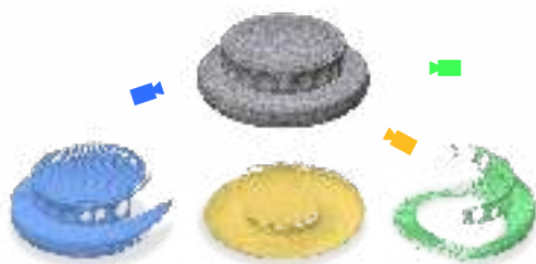
Figure 9: Illustration of the process using Helios++. The input mesh (top) is placed within a simulated scene, where LIDAR sensors (blue, yellow, and green for the example) scan the environment from different viewpoints, each producing a distinct point cloud. The final point cloud is obtained by merging these outputs.
