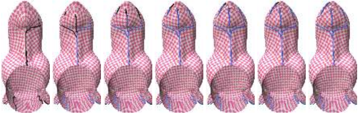
Figure 7: Results after multiple runs of our algorithm. This enables us to capture some natural cuts that our algorithm may have missed. After a few runs cuts our method converges, and the cuts stop expanding.
