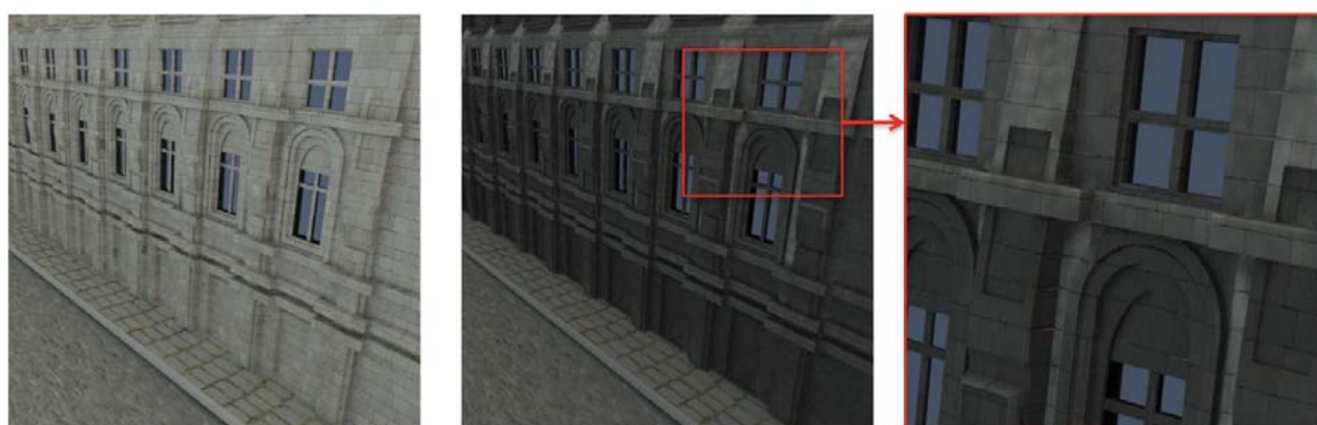
Figure 10: A zoom on different patterns automatically detected on the front of a building (the left image is the clean building, for reference). Rain accessibility, porosity variations and strong flows are clearly observable.
