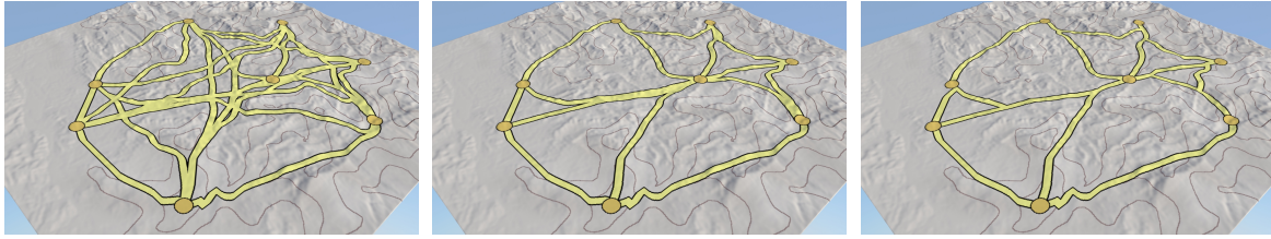
Figure 6: Overview of the road network generation algorithm for a given road type: the complete graph connecting cities (left), the generated proximity graph (center) and the final road network obtained after merging the close parts of the different road paths (right).
