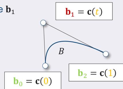
$$\begin{pmatrix} 0 & 0 & 1 \\ t^2 & t & 1 \\ 1 & 1 & 1 \end{pmatrix}^{-1} = \begin{pmatrix} \frac{1}{t} & \frac{1}{t^2-1} & \frac{1}{1-t} \\ -\frac{1+t}{t} & -1 & \frac{t}{t-1} \\ 1 & 0 & 0 \end{pmatrix}$$
