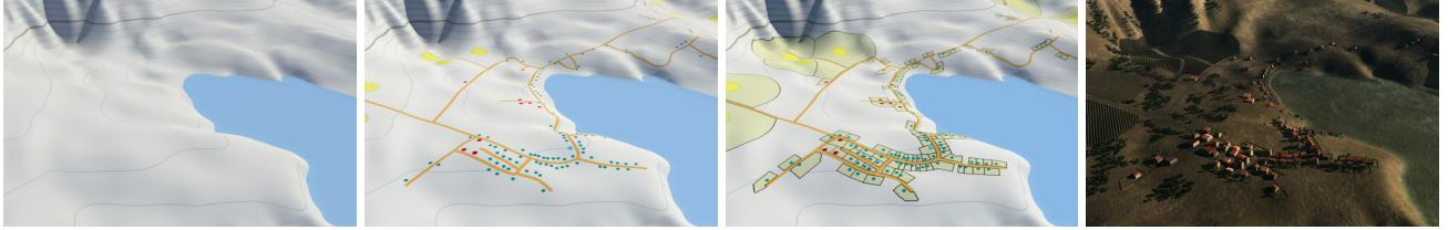
**Fig. 2** Overview of our method: given an input terrain, we first generate the skeleton of the village (roads and settlement seeds), then we add parcels to the village layout, and finally generate 3D geometry for houses.
