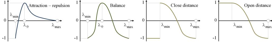
**Fig. 4** Functions used to compute interests. From left to right: Attraction-repulsion function (sociability and worship), balance function (roads and slope), close distance function (water), open distance function (fortifications).
