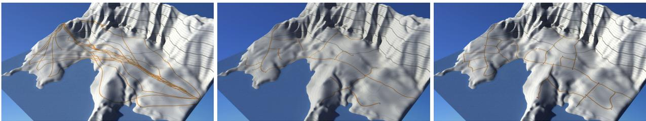
**Fig. 6** Creating new roads. From left to right: without and with road re-use, with road cycle generation.
