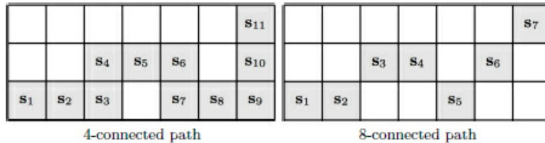
Fig. 1.9 4- and 8-connectivity in a lattice.
