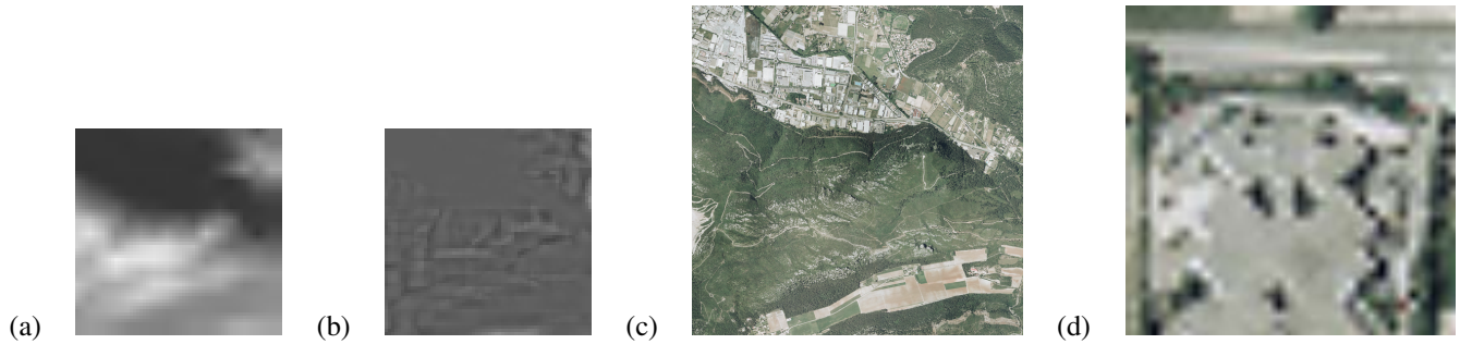
Fig. 10: Reconstruction of the images from the approximation image at Level 2; a) Extracted altitude, b) Difference image between the original altitude and the extracted one, c) Texture, d) Magnified part of texture corresponding to Fig. 7.c.
