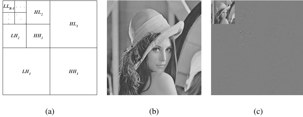
Fig. 2: DWT; a) Subband structure, b) Lena, c) Lena at level 2 DWT decomposition.
