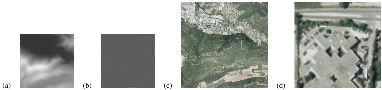
Fig. 9: Reconstruction of the images from the approximation image at Level 1; a) Extracted altitude, b) Difference image between the original altitude and the extracted one, c) Texture, d) Magnified part of texture corresponding to Fig. 7.c.
