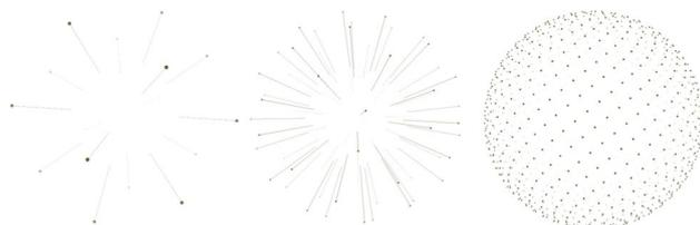
**Fig. 9** Fibonacci sphere sampling. Left:  $nv = 16$  samples with view directions. Center:  $nv = 128$  samples with view directions. Right:  $nv = 1024$  samples to better visualize the sampling distribution
