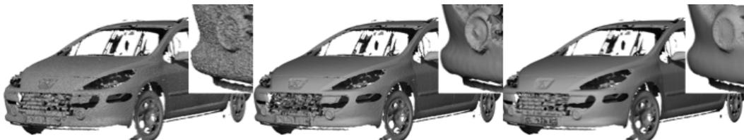
**Fig. 2.10:** Denoising of a data set acquired with a range laser scanner (left: original, middle: similarity-based denoising, right: bilateral filter). In the sparsely sampled area in front of the car, similarity-based denoising tends to create spurious artifacts.
