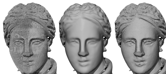
Figure 3: The unmerged head with aliasing artifacts (left), its smooth base (middle) and the merged result (right)
