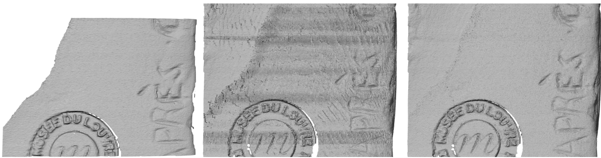
Figure 10: Comparison of a rendering of a single scan (ground truth) and the merging of all scans that overlap in the same region. (Left: ground truth, middle: joint mesh of all scans without merging, right: joint mesh with merging)
