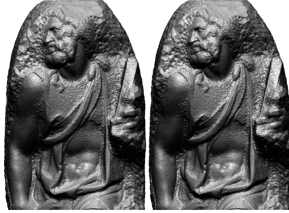
Figure 6: Rendering of the original (left) and decompressed Stanford St Matthew (right), both have 93.4 million points. R = 3\text{mm} , N_{bins} = 16
