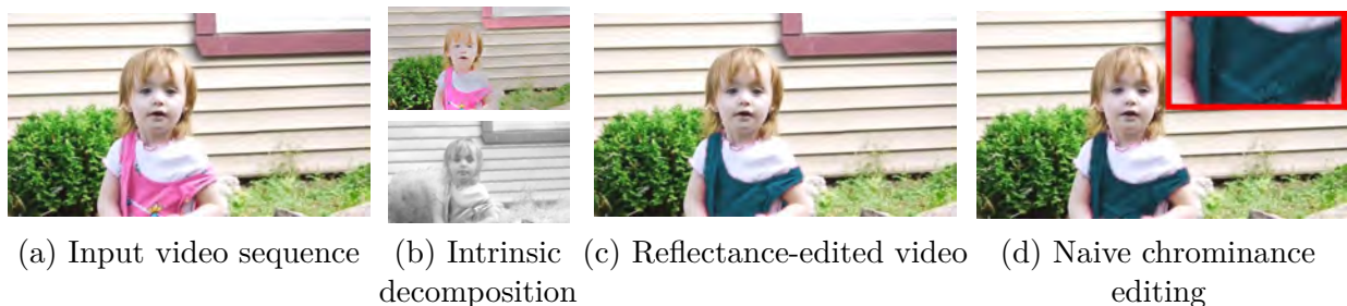
Figure 3.19: Our decomposition enables easy reflectance editing such as re-coloring the girl's t-shirt. By separating the two components, we are able to make these edits while retaining the original illumination in the video. A naive editing of the chrominance leaves luminance variations due to the illustration on the shirt.
