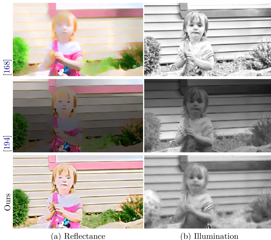
Figure 3.13: We compare our technique (third row) to the decompositions of Shen et al. [168] (first row) and Zhao et al. [194] (second row). Shen et al. has brushes and takes 6 min. while Zhao et al. is automatic and takes 6 s. Our method takes 0.5 s per frame, and provides a more satisfactory decomposition for our applications.
