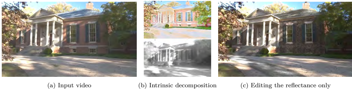
Figure 3.9: A video sequence (a) is interactively decomposed into temporally consistent components for reflectance (b, top) and illumination (b, bottom). Now, editing the textures in the reflectance image does not affect the illumination (c): changes to the brick walls, the roof tiles, and the pathway all maintain the complex illumination of the light through the trees.
