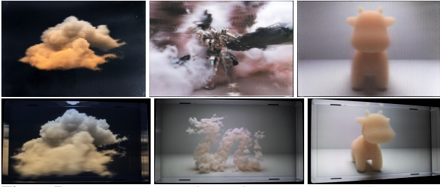
Figure 7: Top row. We print lenticular images using 10 views. Bottom row. Our lightfield display renders images consisting of 45 views. We demonstrate our method on 3 lightfield images.
