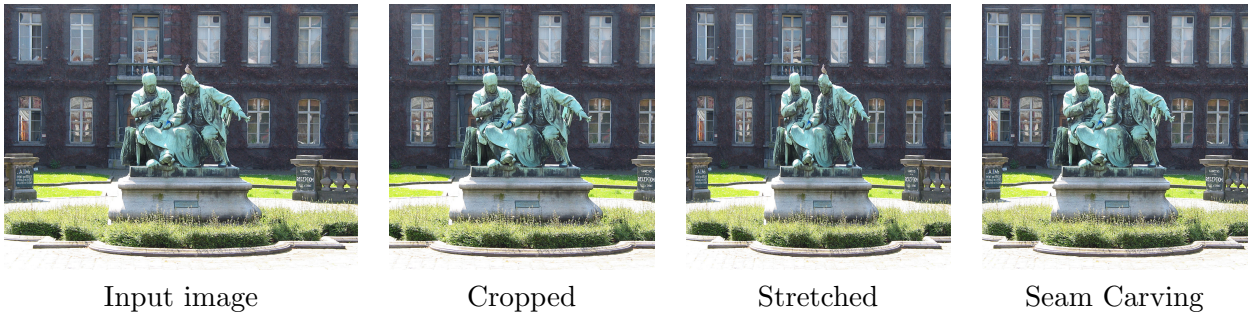
Figure 3.5: Image Retargeting. We would like to make the input image square. Cropping can lose useful information or, like here, the image composition. Stretching, here, distorts the sculpture. The Seam Carving approach removes vertical seams that are least useful. It here removed 450 vertical seams on a 1800x1350 image. The seam carving result was computed in 22 seconds and less than 50 lines of C++ code. Image by Jean-Pol Grandmont, CC-BY 3.0.
