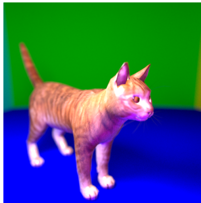
Figure 2.42: I rotated the cat around the vertical axis by 45 degrees using matrix transforms (along with a hardcoded translation), and rotated the camera by -10 degrees around the x axis.
