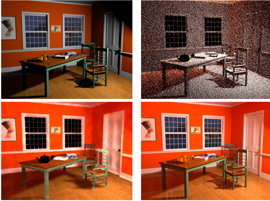
Figure 2.48: Interior scene: (a) Traditional ray tracing. (b) Photon map. (c) Precomputed radiance estimates at 1/4 of the photon positions. (d) Complete image with direct illumination, specular reflection, and soft indirect illumination. Fig. 5.2 of the SIGGRAPH 2002 course “A Practical Guide to Global Illumination using Photon Mapping”.
