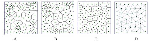
**Fig. 3.** A: Voronoi diagram of a random pointset **X** (black dots), and centroids of the Voronoi cells (green dots). B: configuration after one iteration of Lloyd relaxation. C: after 100 iterations. D: Delaunay triangulation.
