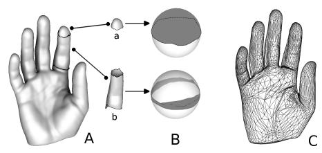
**Fig. 6.** A: a surface with two highlighted zones (a and b). B: the Gauss map of zones a and b (dark gray). Zone a covers half of the sphere, whereas zone b only covers an annulus around the equator of the sphere. C: an isotropic meshing in Gauss space mapped back into Euclidean space is a curvature-adapted anisotropic mesh. Zone a contains more vertices than zone b since it covers a larger space in the Gauss map.
