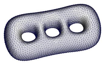
Fig. 2. A Restricted Voronoi Diagram with the associated Restricted Delaunay Triangulation superimposed.
