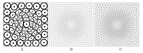
Fig. 4. Anisotropic Voronoi Diagram and Delaunay Triangulation. A: prescribed anisotropy field; B: anisotropic Voronoi diagram and C: Delaunay triangulation.
