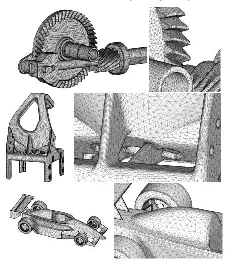
Fig. 8. Anisotropic meshes - mechanical parts.
