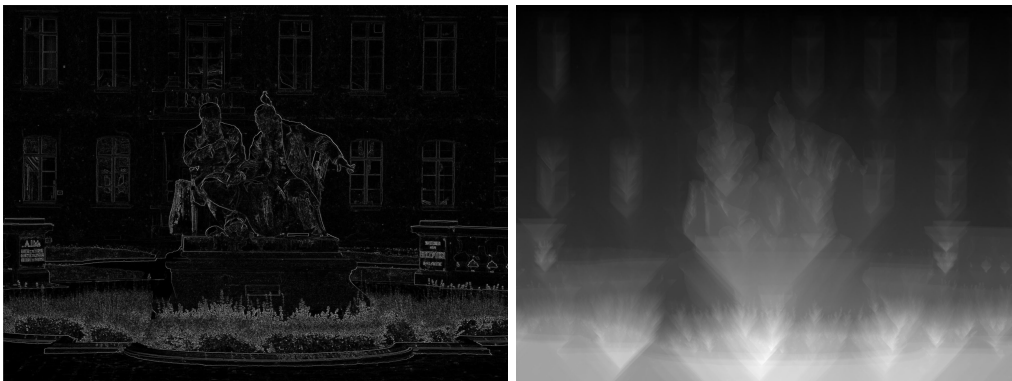
Figure 3.6: From the energy (left) we compute the cumulative energy (here, y = 0 is the top row).
