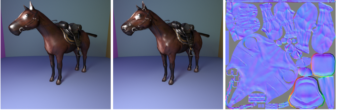
Figure 2.43: Horse model without (left) and with (middle) normal mapping ; the normal map of the body is illustrated on the right. The code is about 850 lines and runs in 1min 12s (left) or 1min 15sec (right) using 1000spp and 5 bounces. The mesh has only 5333 polygons, but normal mapping makes it look more complex. The mesh can be downloaded here: http://www.cadnav.com/3d-models/model-46223.html . It has been rotated like the cat, scaled by 0.15 and translated by (10, -10, 0). The order of the textures to be loaded (since there is no .mtl file) is: body2.d.tga , body2.d.tga , gear.d.tga , gear.d.tga , body2.d.tga . Specular maps were not loaded for these renderings.
