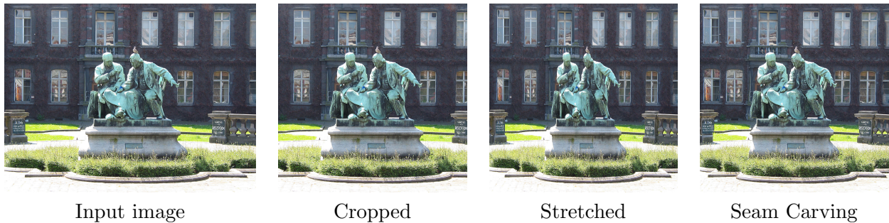
Figure 3.4: Image Retargeting. We would like to make the input image square. Cropping can lose useful information or, like here, the image composition. Stretching, here, distorts the sculpture. The Seam Carving approach removes vertical seams that are least useful. It here removed 450 vertical seams on a 1800x1350 image. The seam carving result was computed in 22 seconds and less than 50 lines of C++ code. Image by Jean-Pol Grandmont, CC-BY 3.0.
