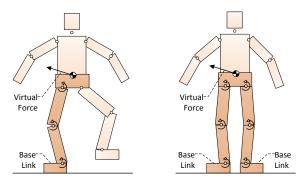
**Figure 2:** Virtual forces applied to the center of mass, through a chain of linked bodies, for single stance (left) and dual stance (right).
