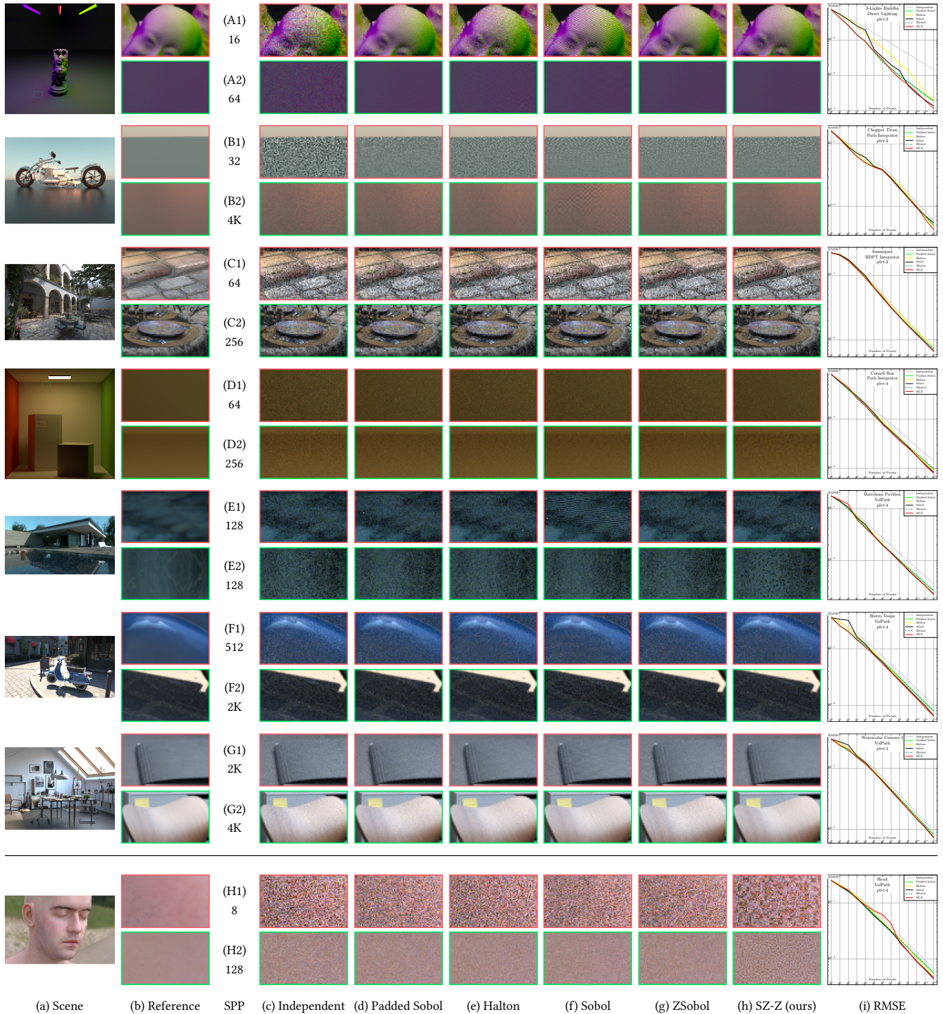
Fig. 6. Example renderings comparing sampling with Z-indexed SZ sequence (SZ-Z) to different state-of-the-art samplers. Specifically, it combines the dithering functionality of ZSobol at low sampling rates with the faster convergence of high-dimensional samplers like Sobol and Halton. We could, however, handpick a few of occasional instances, e.g., (D2) and (E2), where SZ exhibits some noisy artifacts, as well as an example complete scene of “a failure case”, (H), where SZ-Z is notably inferior, although it still takes over eventually. The complete scenes are available in the supplementary materials, along with a few more examples.
