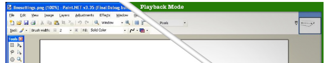
Figure 3. In playback mode, the video is overlaid directly on top of the main application, with a green skin indicating the mode.
