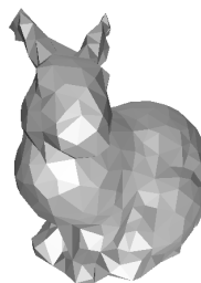
Figure 27: Other aspects of “Bunny” : undersampled data, holes below the Bunny basis (surface with open boundaries)
