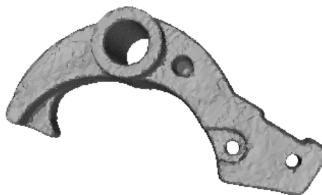
Figure 25: “Meca” (surface without boundary, 12594 points, time 2.638s)
