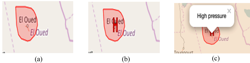
Figure 11 Example of use of multiple representations: (a) geometric, (b) geometric-graphic and (c) geometric-graphic-semantic (see online version for colours)
