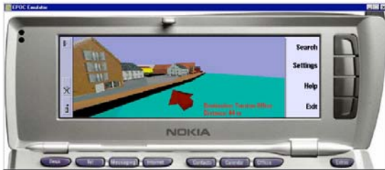
Figure 2: 3D models with Nokia GL on the Communicator 9210. Picture kindly provided by Nokia Research Center, Finland.
