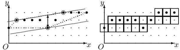
**Figure 3.** The optimal bounding line  $\mathcal{D}(1, 6, 0, 11)$  (squares) of a blurred segment  $\mathcal{S}$  (black disks) of width  $\nu = 2$ .
