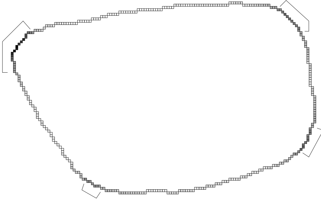
Fig. 6. The radius of curvature is computed for each pixel. The darker the pixel, the smaller the radius of the curvature. Only pixels whose radius of curvature is less than the radius of the largest inscribed circle, are taken into account in the roundness calculation. The roundness is the ratio between the average of the radius of curvature of retained pixels (28.5) and the radius of the largest inscribed circle (40.6), that is 0.70.
